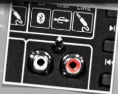
To allow for easy connection to 'consumer' level devices, TOURUS features standard domestic stereo RCA inputs.
